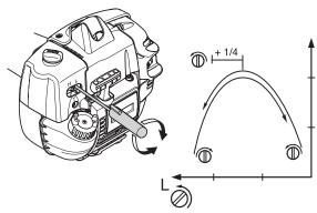
**CAUTION!** If the cutting attachment rotates when the engine is idling the idle adjustment screw T should be turned anti-clockwise until the cutting attachment stops.
