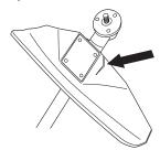
Check that the trimmer head and trimmer guard are not damaged or cracked. Replace the trimmer head or trimmer guard if they have been exposed to impact or are cracked.
