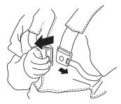
Check that the harness straps are correctly positioned. Once the harness and machine have been adjusted, check that the harness quick release works correctly.
