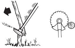
To fell to the right, the bottom of the tree should be pushed to the left. Tilt the blade and bring it diagonally up to the right. Cut with the area of the blade between
