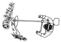
If the blade is angled to the left when clearing grass, the grass will collect in a line, which makes it easier to collect, e.g. by raking.
