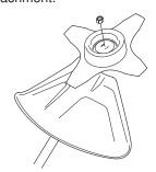
When fitting, tighten the nut in the opposite direction to the direction of rotation of the cutting attachment. To remove it, undo the nut in the same direction as the cutting attachment rotates. (CAUTION! The nut has a left-hand thread.) Tighten the nut using the socket spanner.
