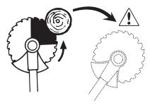
To fell to the left, the bottom of the tree should be pushed to the right. Tilt the blade and bring it diagonally down to the right, exerting firm pressure. At the same time push the stem using the blade guard. Cut with the area of the blade between 3 o'clock and 5 o'clock. Apply full throttle before advancing the blade.
