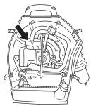
The muffler is equipped with a special spark arrestor screen. The spark arrestor screen should be cleaned once a month. This is best done with a wire brush.
