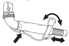
Connect the intermediate pipe and air nozzle. Push the pipes together and turn them so they lock in relation to one another.
